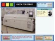
When an error occurs, the location of the error can be shown realistically in a picture.
