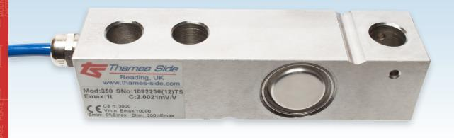
This stainless steel shear beam load cell is fully welded and hermetically sealed to IP68/IP69K, so it can be used in the harshest industrial environments. It is typically used in weigh platforms, tank and vessel weighing, big-bag (FIBC) filling machines and conveyors. The 350i is approved to OIML R60 3000 divisions and calibrated in mV/V/ $\Omega$  by output current matching – which minimises corner correction time on multi-cell platform scales.
