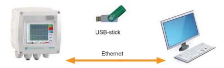
The measured data stored in the data logger integrated in DS 400 can be read-out via USB stick.
