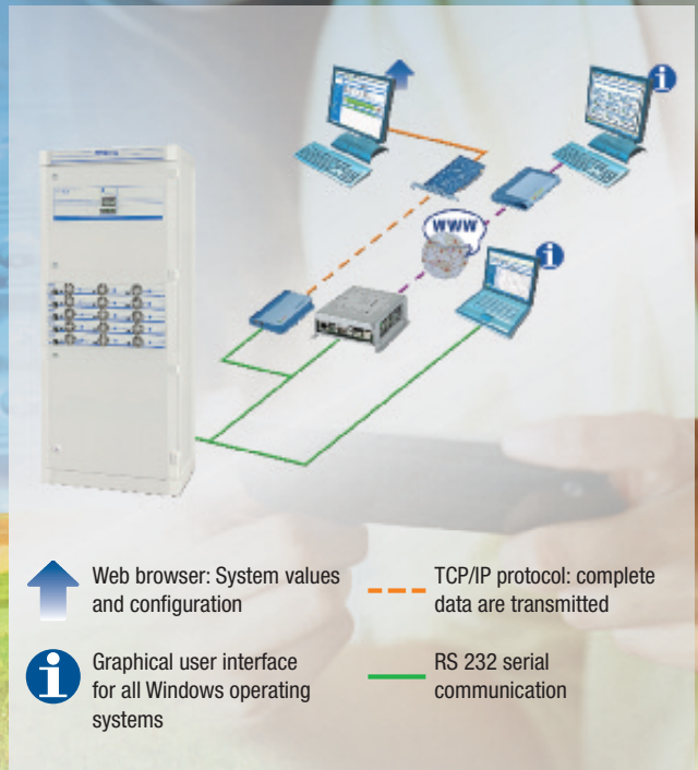
Fig. 9: MCU 2500 remote monitoring system
