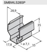
3088063 Snap bracket for mounting WLS28 work lights
