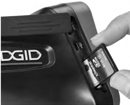
Figure 9 – Inserting the SD Card
