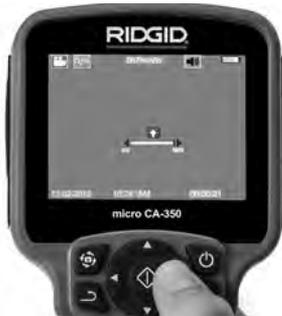
Figure 14 – Adjusting LED
