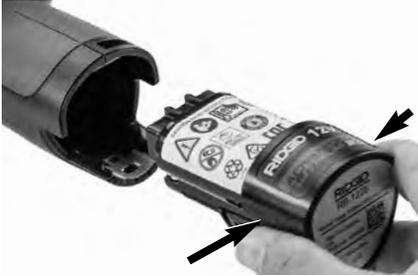
Figure 5 – Removing/Installing Battery
